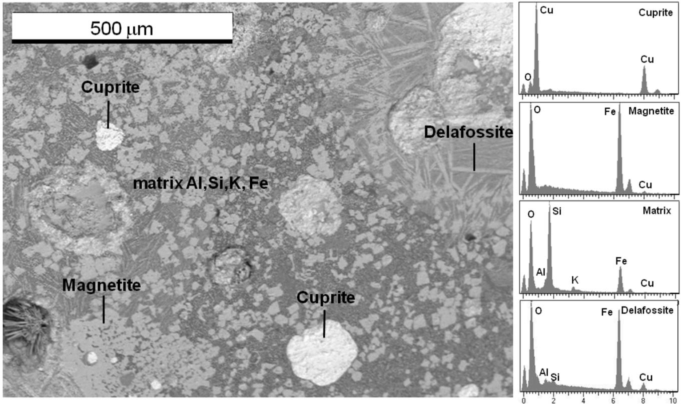
Fig. 5. SEM-BSE image of slag VN301, showing a highly heterogeneous matrix and the identification of cuprite globules, magnetite and delafossite.
