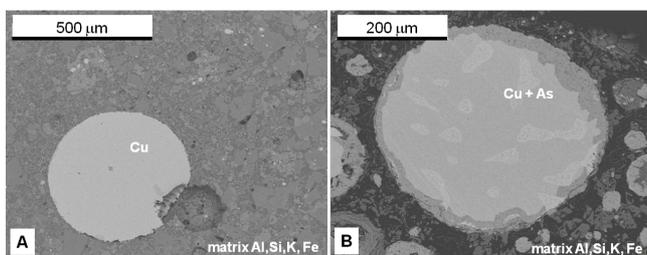
Fig. 6. SEM-BSE image showing the EDS identification of the metallic globule constituents: A:Cu (slag VN309) and B:Cu+As (slag VN313).
