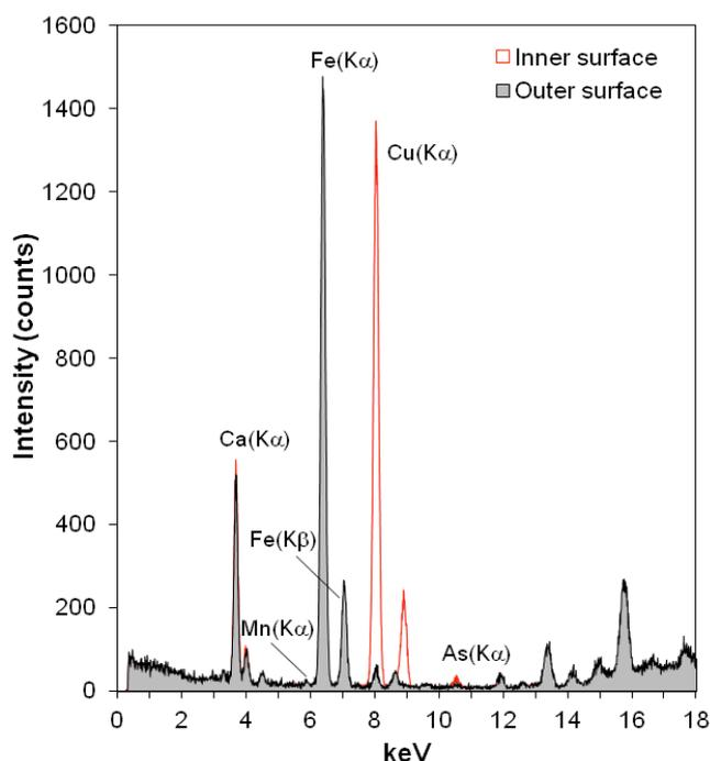
Fig. 4. EDXRF spectrum of the inner surface (red) with visible slag/metallic vestige compared with the outer surface (black spectrum) of VNSP280.
